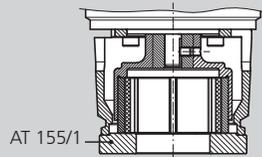
Place the unit vertically on tool **AT155/1** in order to assemble the magnet in the correct position.
