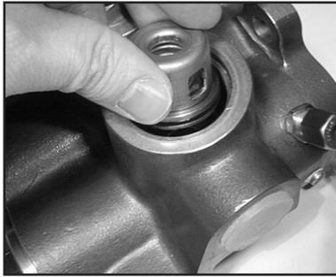
37. Place the entire discharge assembly into discharge port making certain the assembly is properly seated. Install discharge plug (#48) and hand tighten.
