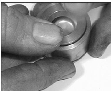
36. Reassemble the discharge valve assembly by placing the valve plate (#45), spring (#46), and spring retainer (#47) on top of the valve seat (#44). Press fit together.
