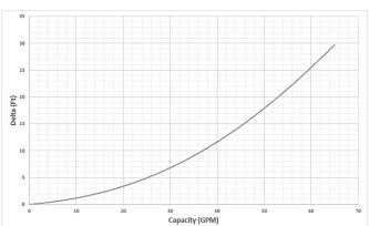
**Note:** Above curve reflects friction loss of the controller as water passes through the controller.
