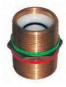
PNC Series are made from PN series cast bronze nipples. A check valve is placed inside to prevent back-flow in plumbing systems. The check valve imposes almost zero flow restriction, and requires less than 1/2 PSI to open. Colored bands indicate flow direction (green to red), confirmed by the permanent laminated tag. Sizes 1/2" to 2". Do not use in diesel fuel or gasoline applications.
