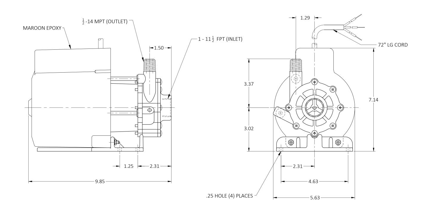
DRAWING SIZE: C-17x22 UNLESS NOTED OTHERWISI ALL DIMS ARE IN INCHES TOLERANCE 0.00 ±0.03 0.000 ±0.005 FRACTIONS ±1/64 PART NAME Dimensional Assy LC-5M-MD 230V 50/60HZ ANGLES ±1°
