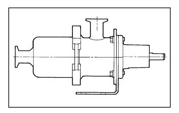
On direct drive units, coupling components should be aligned and spaced at least 1/16" apart.
