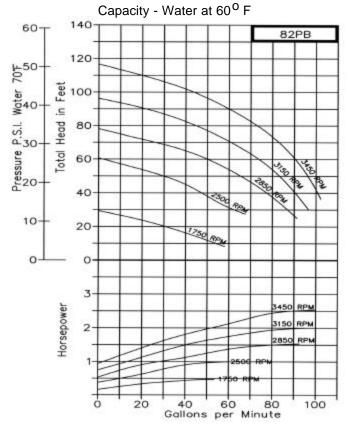
The height of the suction lift should be kept to an absolute minimum and the size of the suction pipe should be equal or larger than the pump inlet port. A foot valve with strainer is recommended a the beginning of the suction line. Self-priming centrifugals must be operated with the shaft in the horizontal position, regular centrifugals may be operated with the shaft horizontal or vertical.
