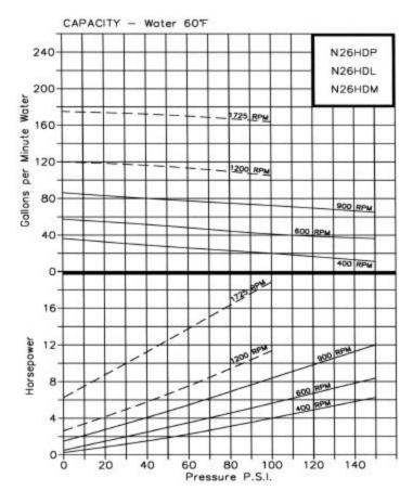
**Note:** Dotted lines(---) recommended for intermittent duty only due to accelerated wear at high speeds and pressures.
