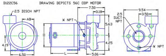
ALL DIMENSIONS IN INCHES. DRAWING REPRESENTS APPROXIMATE PUMP DIMENSIONS, AUTOCAD DRAWING TO SCALE AVAILABLE FROM FACTORY.
