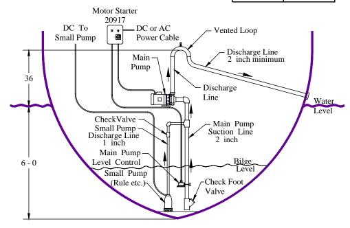
Small pump discharges into suction line of Main Pump, through pump and out the discharge loop and line. Main Pump is always primed and ready.
