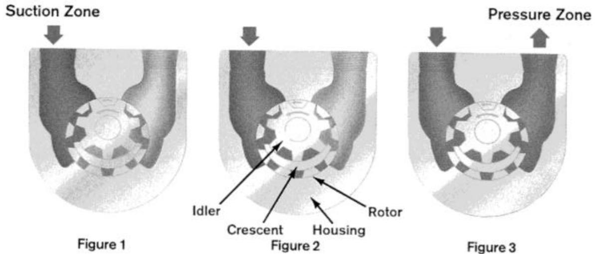
Tuthill Series 4000 cast iron pumps employ the internal gear pumping principle. There are only two moving parts. Pumping action is based on a rotor, idler gear and crescent-shaped partition cast integral with the cover.
