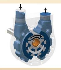
When the teeth mesh on the pressure side, the liquid is forced from the spaces and out through the discharge port.
