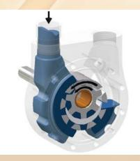
The liquid fills the spaces between the idler and rotor teeth and is carried past the crescent partition through the pressure side of the pump.
