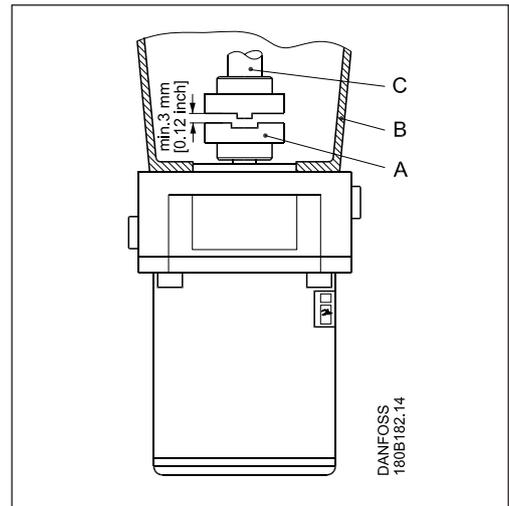
To ensure easy mounting of the flexible coupling without using tools, the tolerances must be dimensioned accordingly.
