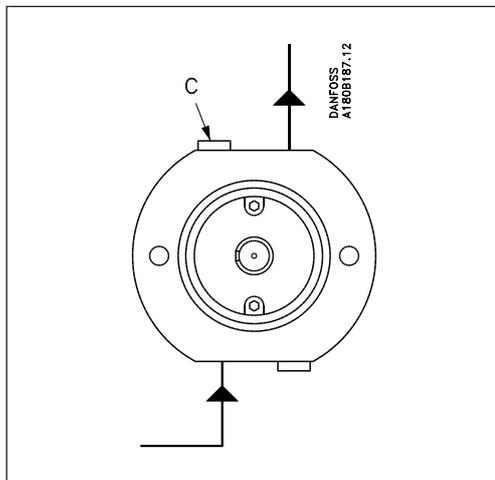
Before starting the pump, the top bleeding plug "C" is loosened. When water appears from the bleeding plug, the pump is filled with water, and the plug is retightened. Make sure that rotation direction of the pump is correct.
