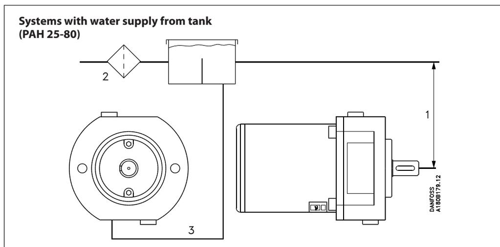
In order to eliminate the risk of cavitation, a positive inlet pressure should always be maintained by observing the following guidelines:
