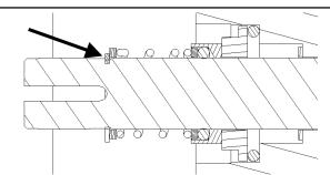
Step 4) Using retaining clip pliers, push retaining clip onto the shaft until you feel it snap into the groove on the shaft.
