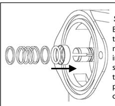
Step 3) Be certain all the components are installed on the shaft. Press them firmly in place using the collar.
