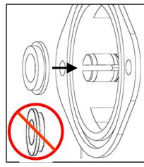
Step 2) Place the tube over the motor shaft, sealend rst as shown. Using the cardboard collar on the tube, push all the seals and other components onto the motor shaft.
