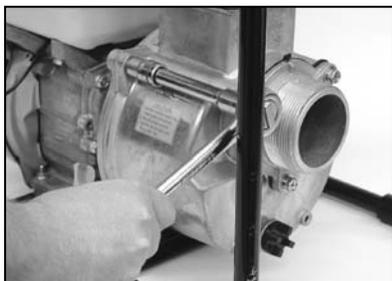
2. Remove volute and inspect for wear. Replace if eroded.
