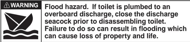
Notice: Before performing any service, disconnect the power supply to the toilet and take precaution to ensure it is not reconnected until the service is complete. Also, pump all water from the toilet bowl and if connected to an overboard discharge, close the discharge seacock.
