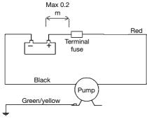
Other electrical devices, eg switch, circuit breaker, must be installed between the pump and the positive (+) lead on the battery (on the red wire).
