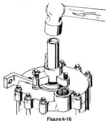
37. Install a bearing lockwasher (#39B) and bearing lock nut (#39B), using the same procedure as on the discharge end.
