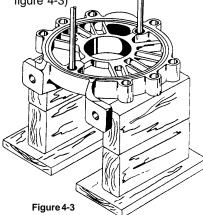
4. Place an "O" ring (#7B) into the groove in the face of the cover (#1B). Slide a left hand channel ring (#10B) onto the guide rods with the water channel facing up.(refer to figure 4-4) With the pump feet in the "six o'clock" position, the large inlet opening should be at "eleven o'clock".
