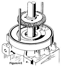
7. Slide a right hand channel ring (#9B) onto the guide rods with the water channel facing downward, toward the impeller.(refer to figure 4-6) The small outlet opening should be in the "one o'clock" position. This completes one stage; a stage consisting of one left hand channel ring (#10B), a right hand channel ring (#9B), and an impeller (#11B) between them.
