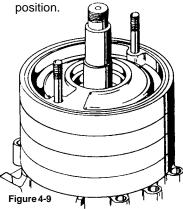
15. Continue installing stages depending on how many stages are in the pump. Don't forget the interstage bushings and the "O" rings (#7B). Remember also to stagger the ring sets to balance radial loads. The odd numbered stages should have openings at the
