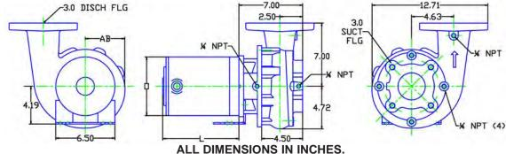
DRAWING REPRESENTS APPROXIMATE PUMP DIMENSIONS, AUTOCAD DRAWINGS TO SCALE AVAILABLE FROM FACTORY
